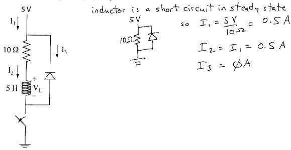
Now the switch is opened. Immediately after the switch is opened, what are the currents  $I_1$ ,  $I_2$ , and  $I_3$ ? According to the sign convention shown for the inductor voltage  $V_L$ , what is the voltage across the inductor right after the switch is opened? What is the rate of change of the current through the inductor,  $dI_2/dt$ ? For all answers, give signs and units.
