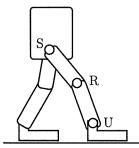
(a) If two feet are in contact with the ground, as shown in the image, and both feet are fixed to the ground (cannot move relative to the ground), how many degrees of freedom does the system have?
