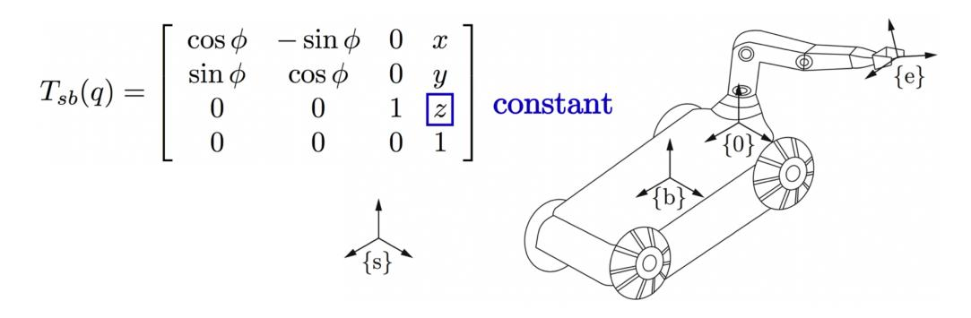
$X(q,\theta) = T_{se}(q,\theta) = T_{sb}(q) T_{b0} T_{0e}(\theta)$
