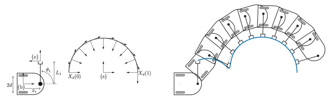
The planar mobile manipulator below has a diff-drive mobile base and a 1R robot arm. Each wheel radius is 0.5. The positive driving direction for each wheel moves the robot forward, and positive rotation for the arm joint is about an axis out of the page. At the configuration below, give the Jacobian  $J_e$ .
