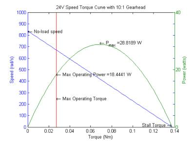
Because the max mechanical power lies outside the continuous operating regime, the power rating for this motor is 18.4 W.
