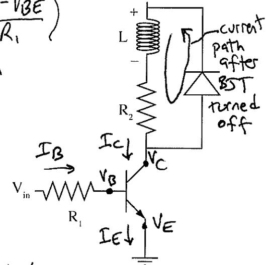
9. Current flows (transistor + LED on) for  $V_{in} > 0.7V$ .
