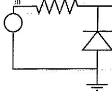
When current flows,  $V_{out} = -0.7V$ .
