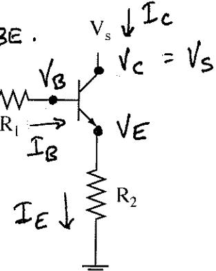
$V_B = 0.7V$ . At saturation,  $V_c = 0.2V$ .
