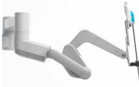
(a) da Vinci S Surgical System instrument arm, © 2016 Intuitive Surgical, Inc.
