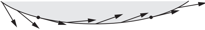
Figure 9.14: A point on the velocity limit curve can only be a part of a time-optimal time scaling if the feasible motion vector at that point is tangent to the curve. A search along the velocity limit curve illustrated reveals that there are only two points on this particular curve (marked by dots) that can belong to a time-optimal time scaling.
