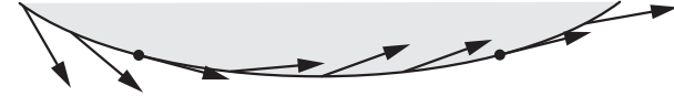
Figure 9.14: A point on the velocity limit curve can only be a part of a time-optimal time scaling if the feasible motion vector at that point is tangent to the curve. A search along the velocity limit curve illustrated reveals that there are only two points on this particular curve (marked by dots) that can belong to a time-optimal time scaling.
