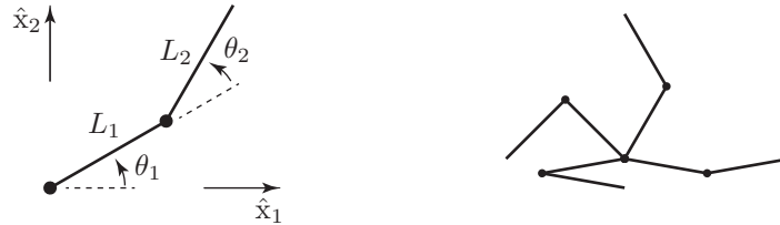
Figure 5.33: Left: The 2R robot arm. Right: The arm at four configurations.
