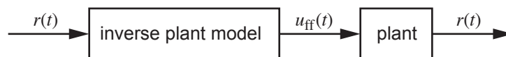
Figure 11.4: An ideal feedforward controller. If the inverse plant model is perfect, the output of the plant exactly tracks the reference r(t) .
