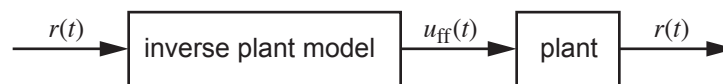
Figure 11.4: An ideal feedforward controller. If the inverse plant model is perfect, the output of the plant exactly tracks the reference r(t) .
