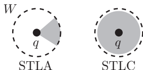
Figure 13.13: Illustrations of small-time local accessibility (STLA) and small-time local controllability (STLC) in a two-dimensional space. The shaded regions are the reachable sets without leaving the neighborhood W .
