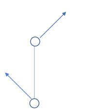
Your mobile robot is equipped with two mouse sensors for odometry. They report the velocity vectors shown. Where is the CoR?
