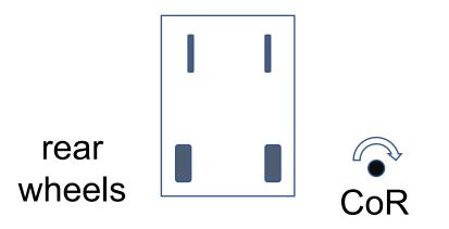
Draw the proper angles of the front wheels of the car-like mobile robot for the CoR shown. (Ackermann steering.) How do the rolling speeds of the rear wheels compare?
