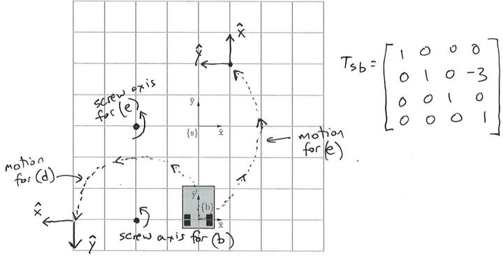
(b) The car's chassis is moving with the twist  $V_b = (0,0,2,0,4,0)^{\intercal}$ . (i) Write the corresponding screw axis  $\mathcal{B}$  expressed in  $\{b\}$  and (ii) in the figure in part (a), indicate the screw axis as a center of rotation (the point the chassis is instantaneously rotating about) along with the sense of rotation (clockwise or counterclockwise).
