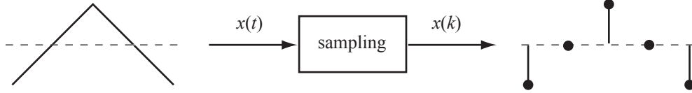
Figure 15.2: The sampling module converts the continuous-time signal x(t) to a discrete-time signal x(k) .
