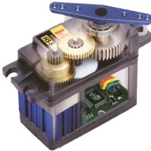
Figure 14.4: An RC servo cutaway showing the gears and the microcontroller that receives the control signal, reads the potentiometer, and implements the feedback controller.
