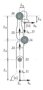
(a) Write the matrix  $M = T_{sb}(0)$  describing the configuration of  $\{b\}$  relative to  $\{s\}$  when the arm is at its home configuration.
