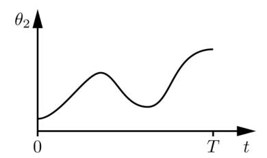
Path: A specification of the configuration as a function of a path parameter.
