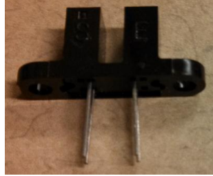
Figure 4: A pre-packaged optointerrupter
