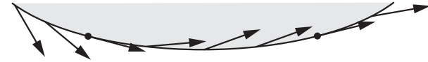
Figure 9.14: A point on the velocity limit curve can only be a part of a time-optimal time scaling if the feasible motion vector at that point is tangential to the curve. A search along the velocity limit curve illustrated reveals that there are only two points on this particular curve (marked by dots) that can belong to a time-optimal time scaling.
