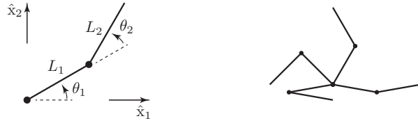
Figure 5.32: Left: The 2R robot arm. Right: The arm at four different configurations.
