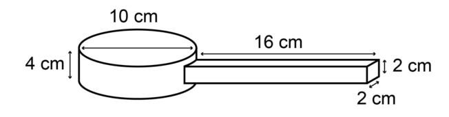
the prism is 1 kg. A frame  $\{a\}$  is defined at the center of the cylinder, with the x-axis along the prism and the z-axis vertical.
