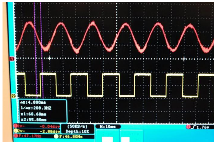
Figure 5: 1-Encoder output before Schmitt inverter, 2-Encoder output after Schmitt inverter
