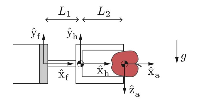
If gravity acting on the apple causes a downward force of 3 N, what is the wrench  $\mathcal{F}_f$  felt at the force-torque sensor due to the apple?
