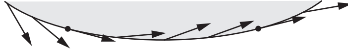
Figure 9.14: A point on the velocity limit curve can only be a part of a time-optimal time scaling if the feasible motion vector at that point is tangential to the curve. A search along the velocity limit curve illustrated reveals that there are only two points on this particular curve (marked by dots) that can belong to a time-optimal time scaling.
