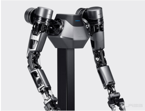
(a) Ambidex arm developed by Naver Labs.
