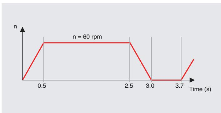
The inertia of load  $J_L$  to be accelerated is 120 000 gcm<sup>2</sup>. The constant friction torque is 300 mNm. The motor is to be driven with the linear 4-Q servo amplifier from maxon (LSC). The power supply delivers max. 5 A and 24 V.
