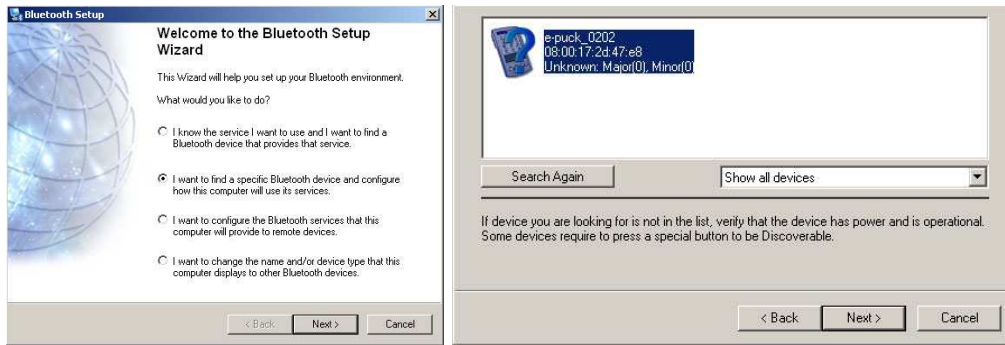
Figure 9: Left: Initial choice on the Bluetooth Setup Wizard. Right: Select your e-puck robot in the bluetooth devices found by your computer.
