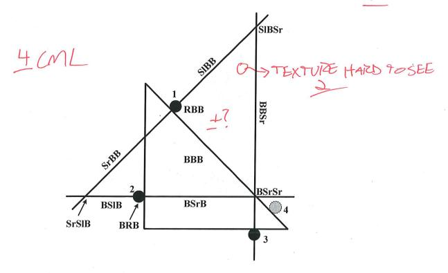
2. The moment-labeling are shown below. The force "Fext" shown in the figure cannot be resisted by the contacts, because after adding this force the moment labeling area are not fully cancelled in the whole plane.
