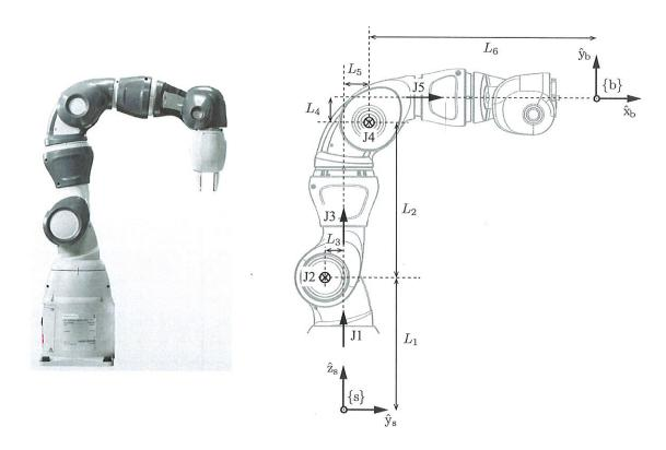
(a) Write the matrix  $M = T_{sb}(0)$  describing the configuration of  $\{b\}$  relative to  $\{s\}$  at this home configuration.
