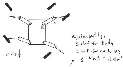
(a) When the robot has no feet in contact with a foothold, how many degrees of freedom does the robot have? Show your reasoning.
