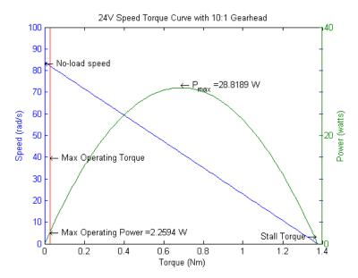
(d) Gearheads are not 100% efcient; some power is lost due to friction and impact between gear teeth. Now assume our 10:1 gearhead from the previous example is  $\eta = 80\%$  efcient. The relation  $\omega_{out} = \omega_{in}/G$  must be preserved (its enforced by the teeth), so we will use the relation  $T_{out} = \eta G T_{in}$ , giving  $P_{out} = T_{out}\omega_{out} = \eta T_{in}\omega_{in} = \eta P_{in}$ . Draw the speed-torque curve for the 24 V motor with an 80% efcient 10:1 gearhead.
