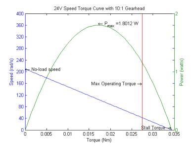
Since the maximum power output for the motor at this voltage lies within the continuous operating regime, the power rating for this motor is 1.80 W.
