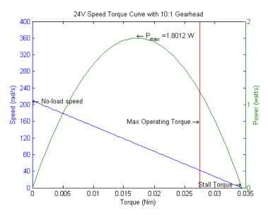
Since the maximum power output for the motor at this voltage lies within the continuous operating regime, the power rating for this motor is 1.80 W.
