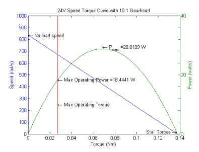
Because the max mechanical power lies outside the continuous operating regime, the power rating for this motor is 18.4 W.
