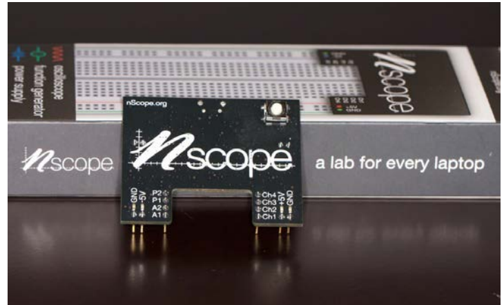
The nScope portable function generator and oscilloscope.
