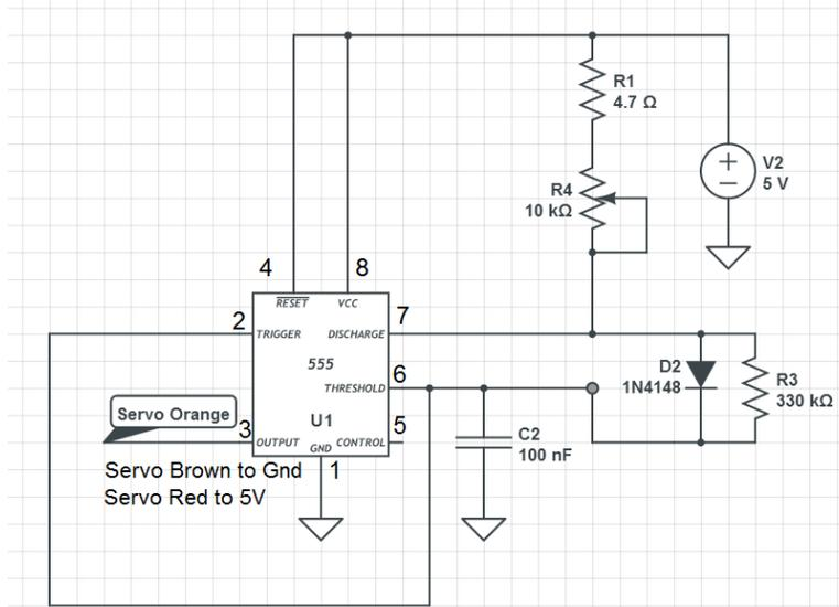
Roughly based on <http://www.555-timer-circuits.com/servo-tester.html>
