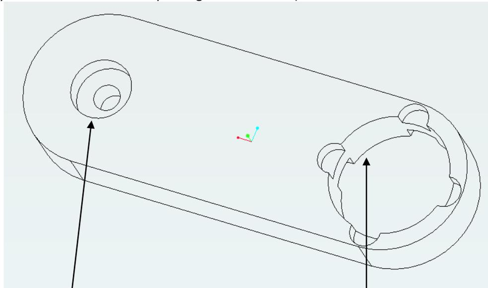
0.195" hole for RC starry shaft, with thru-hole for screw
