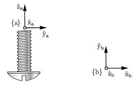
(a) What is the screw axis  $S_a$  corresponding to advancing into a tapped hole? Give a numerical 6-vector.
